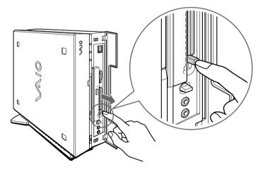
The card is ejected from the card connector. Remove the card by holding it by its edge and pulling it out carefully.
